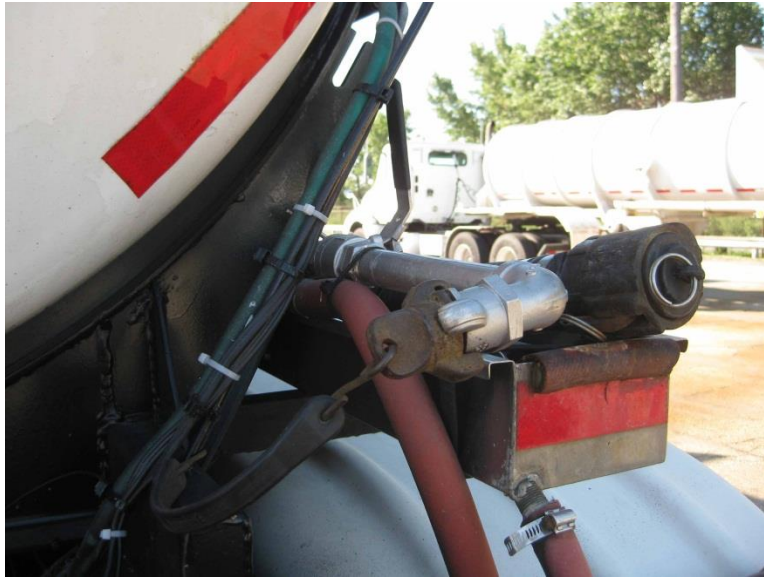
Figure 8 - Air fittings and offloading hoses not protected
