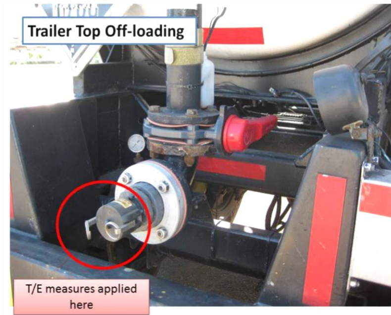
Figure 6- Common off-load point protected; torqued bolts and misc. air fittings are not.
