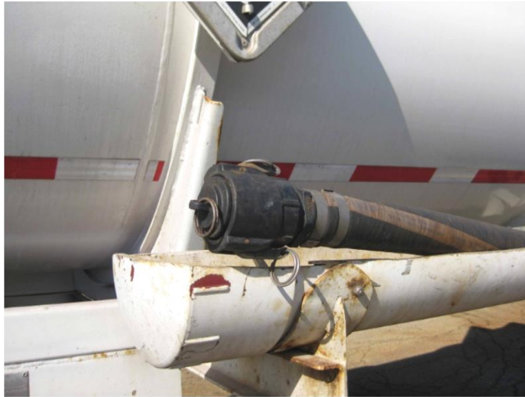
Figure 14 – Off loading hose not protected
