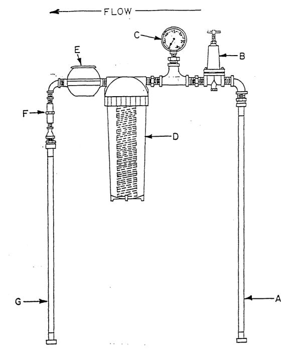
Figure 1. Water Sampling Device
