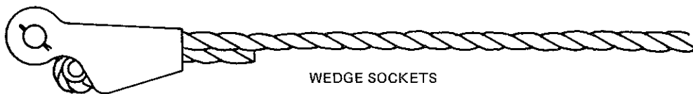
Fig. 29 Wire Rope End Attachments and Drum Anchors Commonly used on Surface Mining Machines
