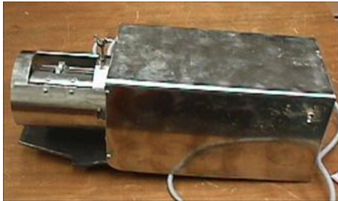
Figure 23 – Mechanical stainless steel oyster grinder
