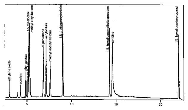
Mix 2: Analytes distilled at 0.25 mg/L, internal standards at 2.5 mg/L
